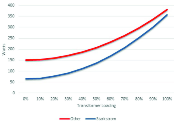
10kVA Transformer: Heat Loss Comparison
